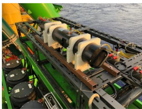
Prototype LISST-RTSSV mounted at the rear of the collector vehicle. Source: Sequoia Sci.
