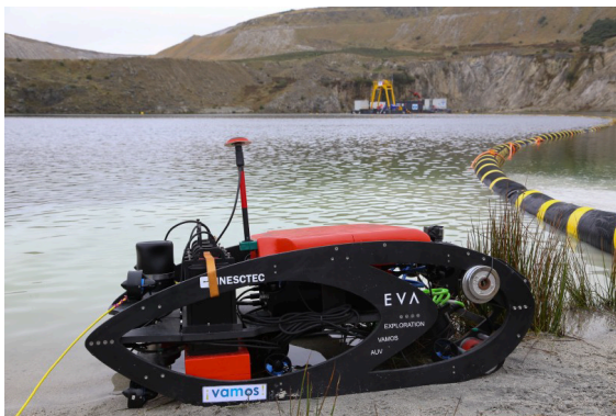
Figure 1. EVA HROV/AUV in tests on Lee Moor Mine, UK Figure 2. VAMOS AUV system architecture
