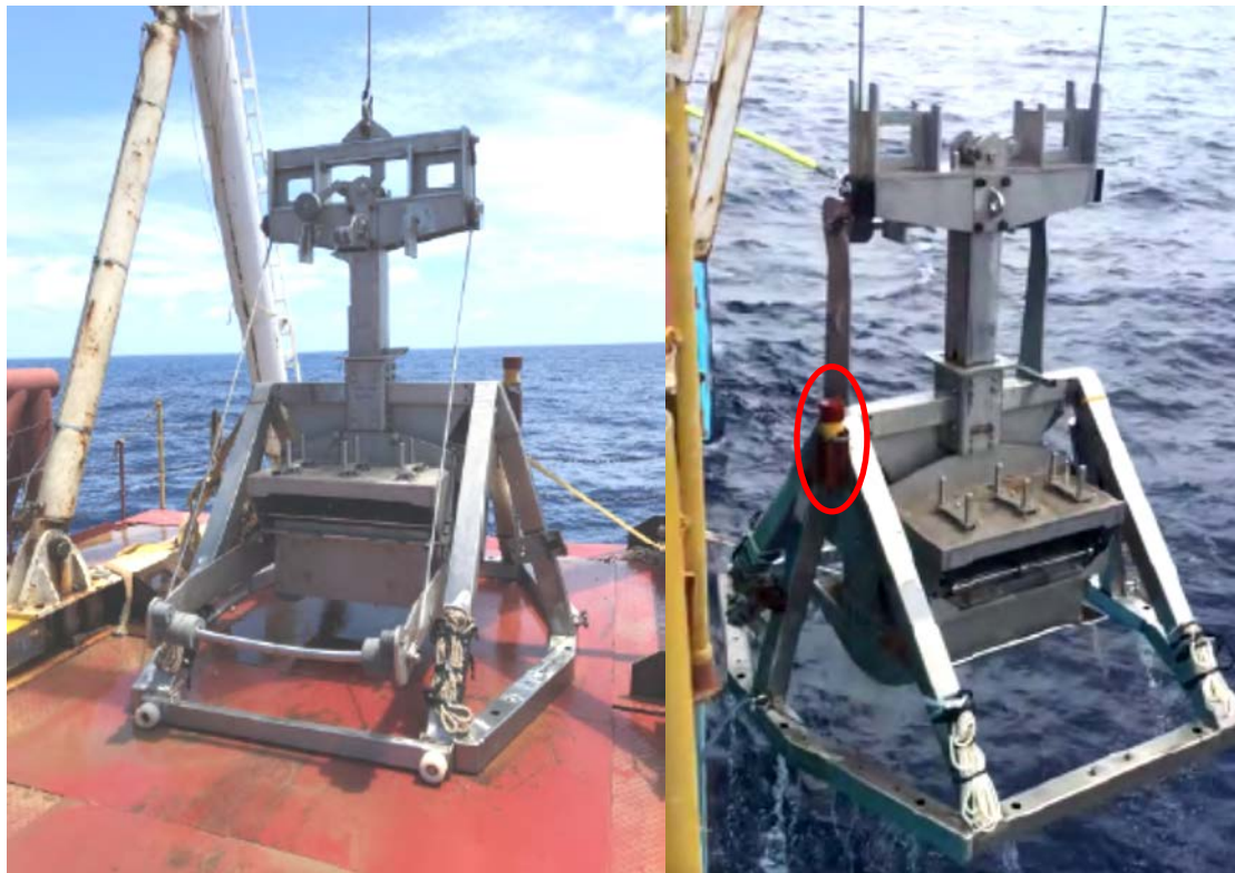
Figure 6. 0.75 m 2 Box Core manufactured by K.C. Denmark A/S used for mineral sampling, geotechnical tests, and opportunistic environmental sampling for NORI D Campaign 3. Photo on right shows USBL transponder attached to box core frame.
